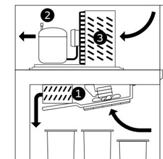
1 Evaporator 2 Compressor 3 Condensing unit
